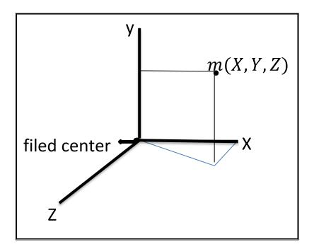
A point such as M is described by distances located in the direction of three perpendicular axes, X.Y.Z. where the M point(X.Y.Z) has a point away from the coordinate center (0) in the direction of the three axes (X.Y.Z).
