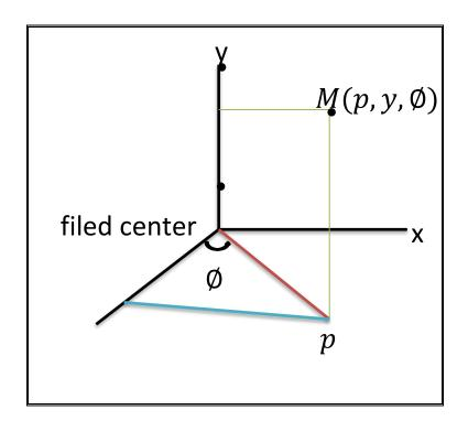
\*Any point such as M is assigned by two distances: (P.y),angle  $(\emptyset)$ confined between the axis(Z) and the  $drop\ of\ the\ line\ P\ (OP)\ in\ the\ level\ (Zy)$
