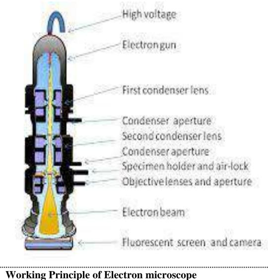
Electron microscopes use signals arising from the interaction of an electron beam with the sample to obtain information about structure, morphology, and composition.
