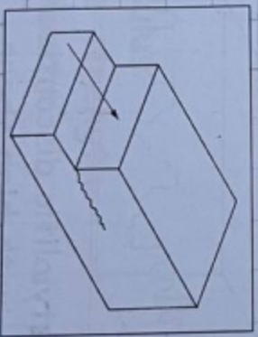
Mode 2 (in-plane shear)
