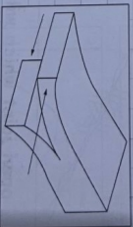
Mode 3 (out-of-plane shear)
