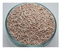
Zeolites are extruded as pellets for easy handling in catalytic reactors.
