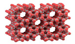
The microporous molecular structure of the zeolite ZSM-5 is exploited in catalysts used in refineries
