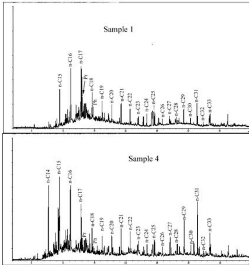
Figure 3. GC-FID chromatograms of saturated hydrocarbons of two samples.
