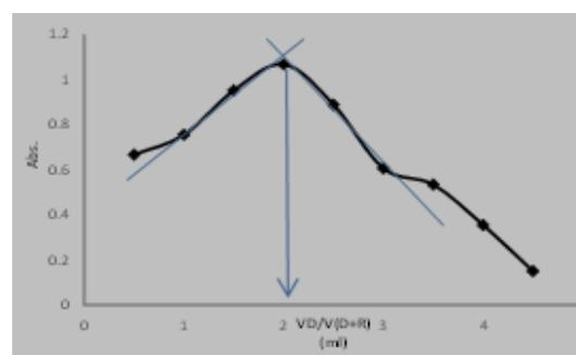
Fig.(10):Continuous variation method of AMP
