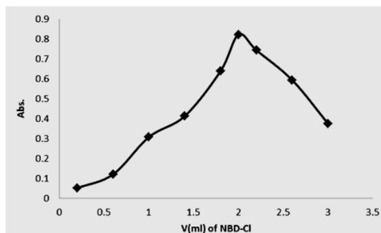
Fig.(5): Effect of vol. of NBD-Cl on AMP-NBD-Cl product
