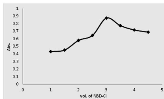
Fig.(6): Effect of vol. of NBD-Cl on LPZ-NBD-Cl product
