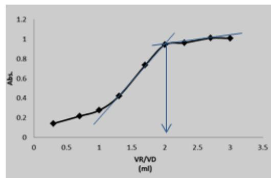
Fig.(9):Mole-ratio method of AMP
