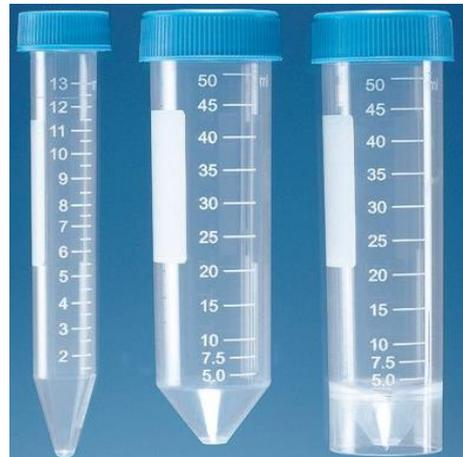
Falcon tube ( centerifuge test tube)
